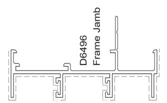
1. Lay Frame parts on a bench or Trestles. Jambs are handed Left and Right (viewed from the outside). Remove the yellow backing on the sill gasket. Make sure the reveal fins line up before screwing the jambs to the head and sill.
